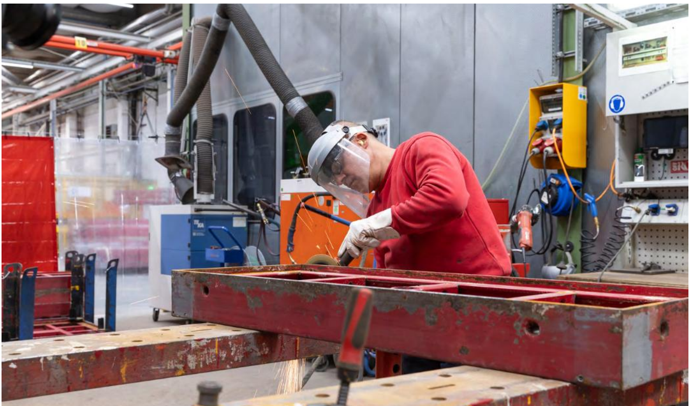
Refurbishment of a PERI formwork element.
