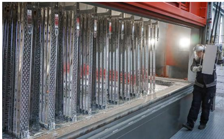
Galvanization of PERI scaffolding production in Günzburg.
