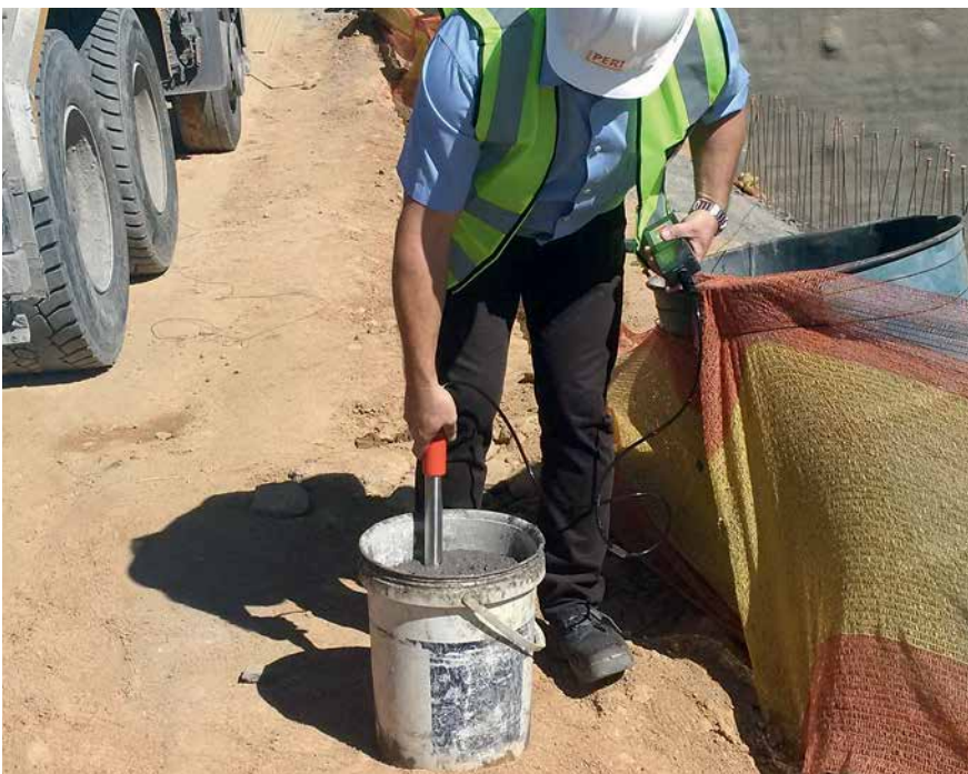
The PERI SONO w/c analyzer consists of a measuring probe and a hand-held transmitter with a display. The fresh concrete measurements are carried out in a common plastic bucket.
