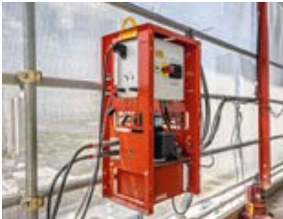
Via light signals on the RCS MAX Hydraulic Unit and via the display, malfunctions are immediately indicated and can thus be quickly detected and easily remedied on site.
