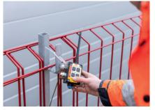
To transmit the measured values, connect the ISC Thermocouples to an ISC Temperature Node. You can attach this almost anywhere, such as to the formwork or a guardrail.
