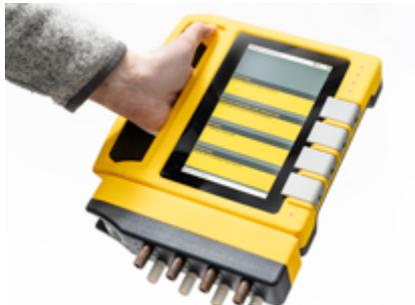
The recorded data is sent to the ISC Hub via the ISC Node. The measurement results are shown immediately on the ISC Hub display.
