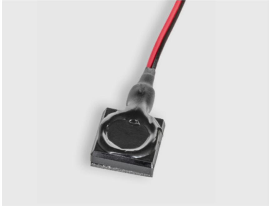
The ISC Concrete Detection Sensor is remarkably easy to install: You can attach it directly to the formwork before concreting. To transfer the measured values, connect the sensors to an ISC Node.
