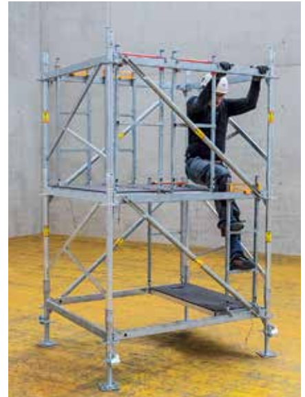
The intermediate guardrail of the Platform MDS can also be used as a climbing aid. The distance is 50 cm on the "red" side and 33 cm on the "yellow" side.
