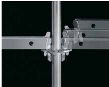
With the ledger assembly, the wedge falls into the opening of the rosette through its own force of gravity and locks automatically. The rosette node connection is extremely rigid with a high loading capacity.
